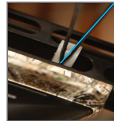
Fig 6.1: "R" Cam Cable Route (View from Right side of rail slide)
