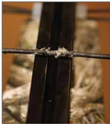
Fig 4.1: Example of a worn crossbow string
