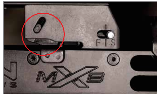
Fig 3.1: Automatic Anti-dry fire mechanism
